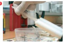
Now attach the static mixer to the cartridge. (This screws in)
