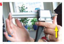
Raise the lever at the rear (see yellow arrow) and push the plunger all the way in, until it stops.
