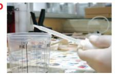
Pull gently on the trigger until resin is ejected from the end of the static mixer. Wipe excess resin from the static mixer.
