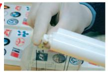
Gently break off the seal of the cartridge. Keep the seal in a safe place for resealing later.
