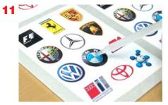
Dome your decals by gently squeezing resin onto the surface. Be careful not to apply too much or too little. (This will come with practise) The resin will automatically move toward the silicon coated backing paper. Don't worry if it doesn't move all the way to the edge of the decal - you'll have time to correct this later.
