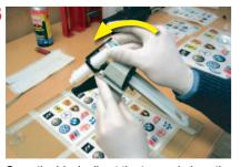
Open the black clip at the top and place the cartridge into the dispensing gun.
