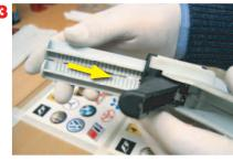
Place plunger into dispenser, ensuring serrated edge faces the handle.
