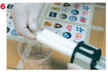
Remove safety cap from the cartridge by turning 90° and gently pulling.
